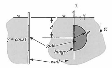
A semicircular gate of radius R, hinged along its vertical, straight edge, is located in a vertical wall bounded on one side by a liquid of constant specific weight  $\gamma$ . The center of the gate is at a depth d below the liquid free-surface.
