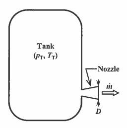
c) How will the mass flow rate change if the tank is filled with more of the same gas, and the tank pressure and the tank temperature both double?
