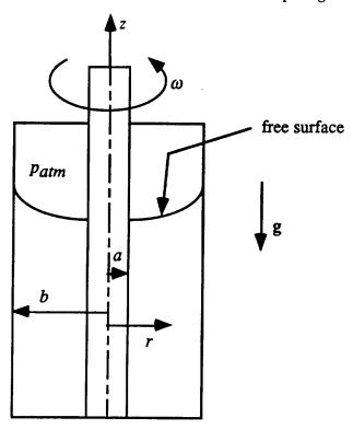
Consider the purely circumferential, steady motion of a Newtonian fluid in the partially filled annular region  $a \le r \le b$  between a rotating inner cylinder and a stationary outer one, as shown above.
