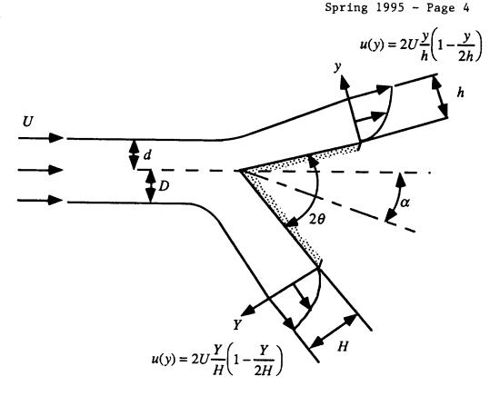
A liquid sheet of thickness d + D strikes a two-dimensional wedge of half-angle  $\theta$  (inclined at an angle  $\alpha$  to the oncoming liquid) with uniform speed U, as shown in the figure above. The nose of the wedge is *not* necessarily in the center of the sheet, i.e.,  $d \neq D$ . The sides of the wedge are long enough that the velocity profiles on each side develop a parabolic shape, as shown in the figure.
