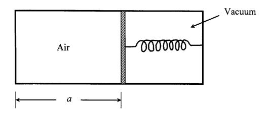
The cylinder initially contains air ( $c_p = 1.004 \text{ kJ/kg} \cdot \text{K}$ ;  $c_v = 0.717 \text{ kJ/kg} \cdot \text{K}$ ; and  $R = 0.287 \text{ kJ/kg} \cdot \text{K}$ ) at 25 °C, and a is initially at 5 cm. The cylinder walls are then slowly cooled and the piston moves to the left until  $a = a_2 = 4$  cm. Compute the energy transfer as heat from the gas for this process.
