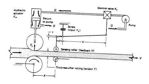
In the above figure, the control valve can be modeled by the following approximation:
