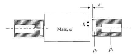
The pocketed-orifice bearing can be modeled as a dynamic system consists of an air capacitor (with pressure  $p_c$ ) and two orifice resistors (a fixed orifice between  $p_s$  and  $p_c$ , and a variable orifice between  $p_c$  and the ambient). You may assume that the flow through the orifice is proportional to the square root of the pressure difference across it.
