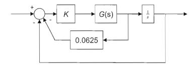
In the velocity-feedback control system shown above, K > 0, and the plant transfer function is
