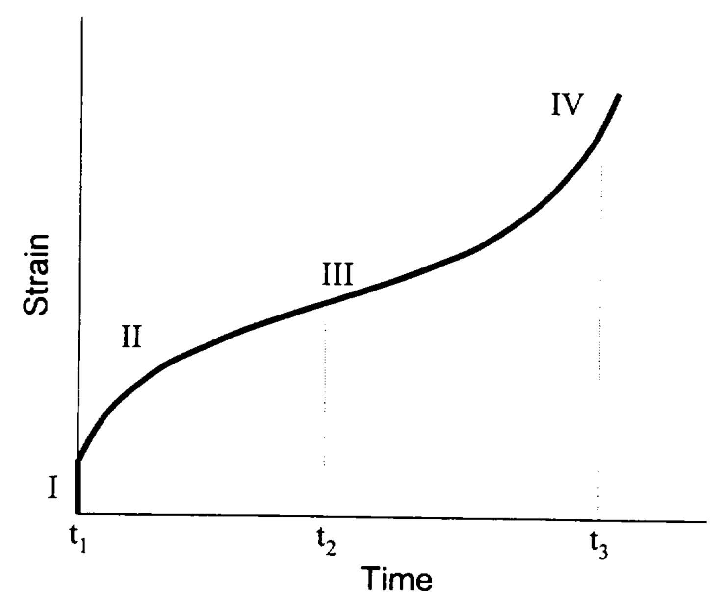
Consider strain vs. time curve for a constant load uniaxial tension test at room temperature.
