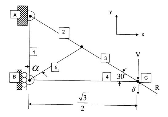
The simple pinned joint truss structure shown above has a fixed pinned joint at "A" and a simply supported pin joint (no horizontal displacement) at "B". Vertical displacement  $\delta$  of the joint at point "C" is affected by applied loads V and R. We limit our consideration to infinitesimal strains in each truss element.
