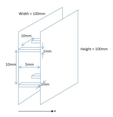
Assume each copper plate is at a uniform temperature. The plate at x=0 is at a higher temperature than the other one which is at the ambient temperature of 300 K.
