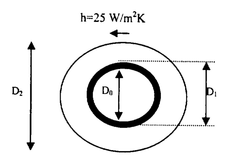
The electrical wire, of diameter  $D_1=10$  mm, has an insulating core of diameter  $D_0=6$  mm, shown above. It is carrying a current of 100 amperes. The insulation of thickness 5 mm ( $D_2=20$  mm). Given that the forced convection coefficient from the external surface is 25 W/m<sup>2</sup>K and the ambient temperature is 20 °C, calculate the maximum internal temperature of the wire.
