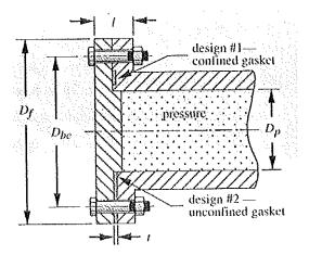
One power source that is being contemplated is compressed air stored in a flanged cylindrical tube (outer diameter = 5.2 inches) sealed off by a lid that is bolted onto the cylinder's flange. In the above figure, a schematic drawing of the tube and its flange and lid is given. The lid is bolted onto the flange.
