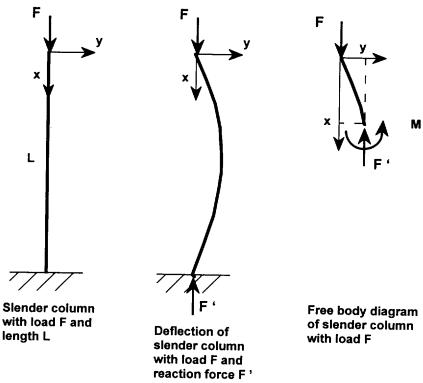
The curvature of such a slender column subject to an axial load F can be modeled by
