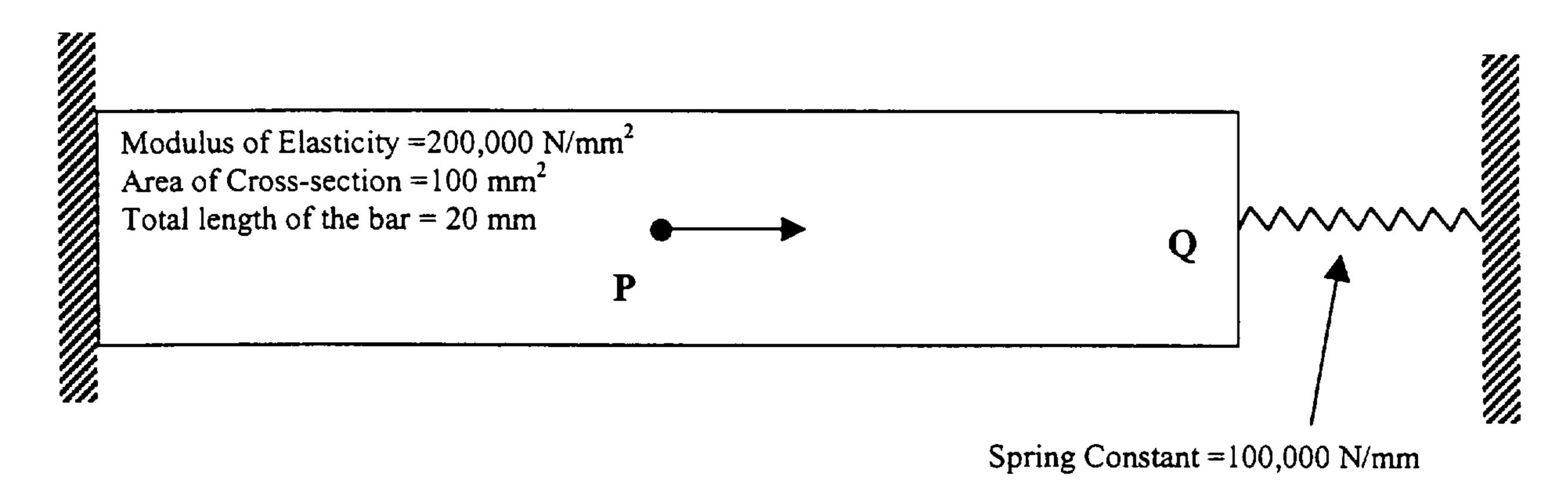
Assume that the whole structure is heated during operation and the temperature of the unit rises by 30 °C. Assume that the coefficient of the thermal expansion of the axial bar is  $12*10^{-6}$   $\checkmark$  °C and that of the spring is negligible.
