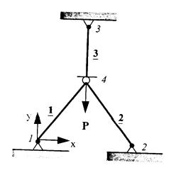
All members are of equal length L, cross-section area A, and made of the same material. The distance between joints 1 and 2 is L.
