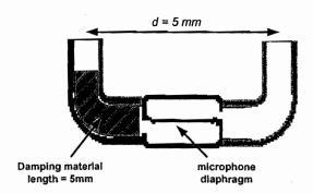
c) Given the distance between sound ports and the length of material in the tube as above, determine the value of R so that the microphone response has a minimum at for sound incidence from the left side (i.e.  $\theta = 180^{\circ}$ ) at f = 1 kHz. The properties of air are  $\rho_o = 1.21 \text{ kg/m}^3$ , and  $c_o = 343 \text{ m/s}$ .
