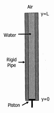
Consider a water-filled rigid-walled pipe of length L with a piston at one end (y=0) and open to the air at the other end (y=L). At time t=0 the piston starts moving upward at some small velocity  $v_o$  and continues to move with this velocity indefinitely. (Assume that the velocity is sufficiently small so that, for the purpose of establishing boundary conditions, the piston can always be considered to be located at y=0).
