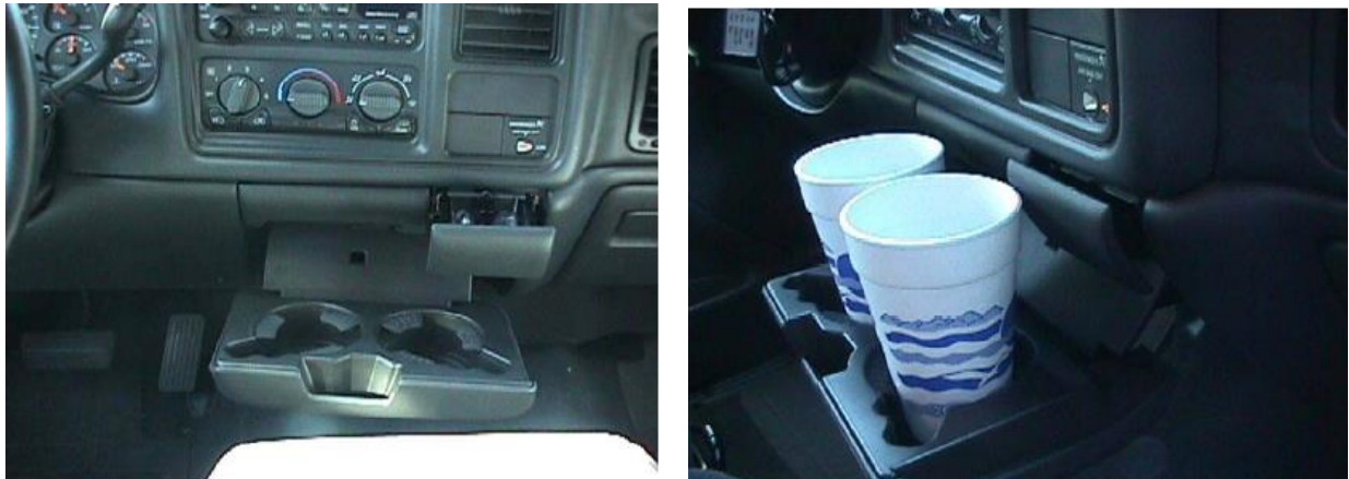
Figure 1(a): 1999 Model-Year GM Silverado cup-holders and ashtray on the instrument panel with cups in cup-holders
