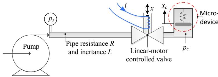
For high-bandwidth design, the rotor dynamics of the linear-motor (which can be modeled as a translational mass-damper-spring system) and the pipe inertance must be taken into account.
